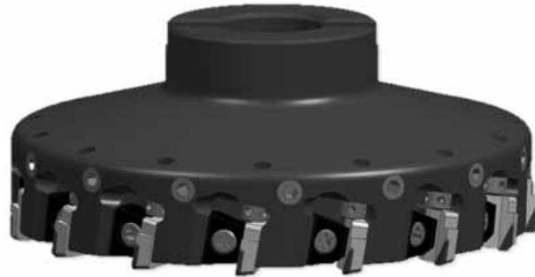
The HF-PCD Cutter for aluminum is a special designed steeled-body cutter. It is utilized to achieve high-efficiency machining with easy fine adjustment, easy-to-use wedge-type insert clamp and anti-fly out mechanism.
